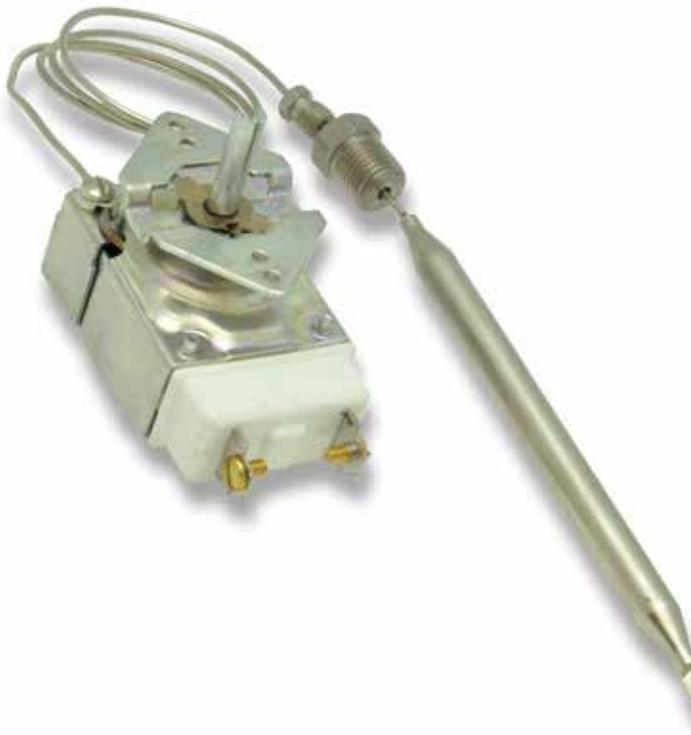
The Robertshaw® RX series is a single pole single throw (SPST) thermostat designed for today's demanding Millivolt/Milliamp direct current applications. The RX thermostat features a hermetically sealed reed switch to provide durability and accuracy in the harshest environments.
