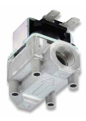
The Robertshaw® SGV valve has a rugged design which exceeds current qualifications. Its function is to control the flow of gas in an appliance application. Die cast aluminum bodies with multi-position, rigid mounting and standard brackets are available. This gas solenoid valve can be used for a wide variety of applications, especially in ovens and griddles.
