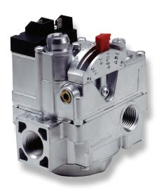
The Robertshaw® 720 Series 24 Volt Dual Gas Valve is a six-function gas valve incorporating a manual valve, safety shut-off magnet, dual automatic valves, main gas regulator, and pilot adjustment. Models are available with and without a pressure regulator. Uni-Kit® models are factory set at 3.5" WC for natural gas, but can be converted to LP by installing the regulator conversion kit included.
