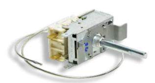
The Ranco® K Series Temperature Controls are used globally to control the temperature in commercial and residential refrigeration, air conditioning and heating applications. The K Series Temperature Control is a cycling thermostat with a single pole single throw (SPST) close-on rise switch and narrow differential for custom applications.
